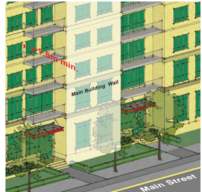
Figure 6-86: Preferred location of two-sided balconies
