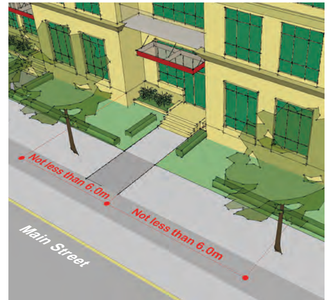
Figure 6-82: Width of wall panels for residential frontage
