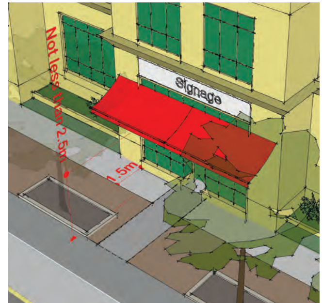
Figure 6-78: Provide weather protection along retail edge
