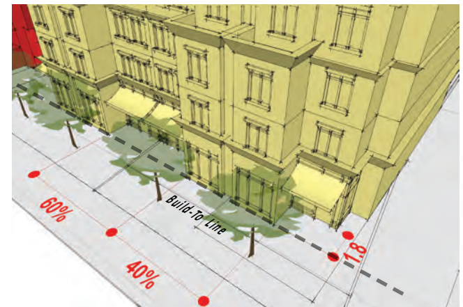
Figure 6-41: Articulated Street Edge
