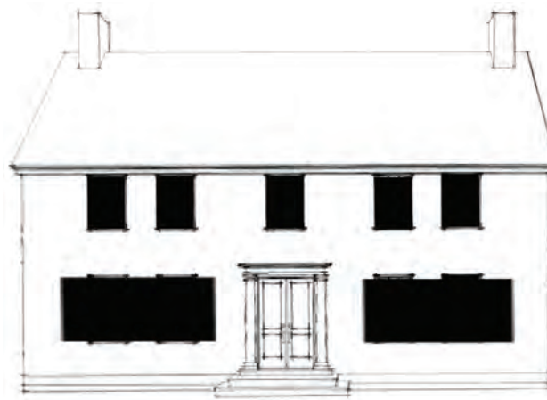
Figure 6-24: Inappropriate Window Size and Ratio
